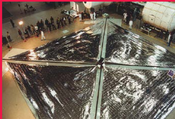
↑ ESA/DLR Solar Sail full-scale deployment test, 20 x 20 m, in 1999 (ESA/DLR)
