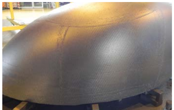
↑ IXV nose thermal protection (Herakles)
