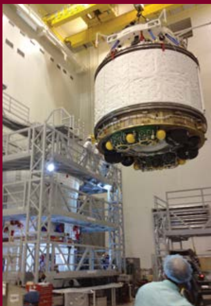
Mating of ATV-4 Cargo Carrier and Service Module in progress
