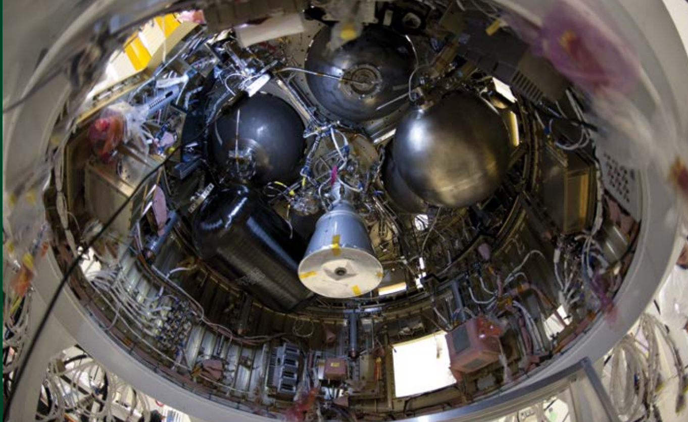
↑ View inside the Attitude and Vernier Upper Module, a reignitable liquid-propellant fourth stage containing the avionics that serve as the 'brain' of the vehicle
